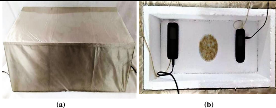
Figure 3: (a and b): Shielded chamber for RF electromagnetic radiation exposure
