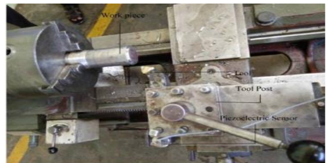
Fig.No.3 Piezoelectric Sensor on the tool post
