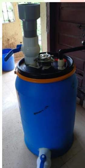
Fig-3 image of the digester
