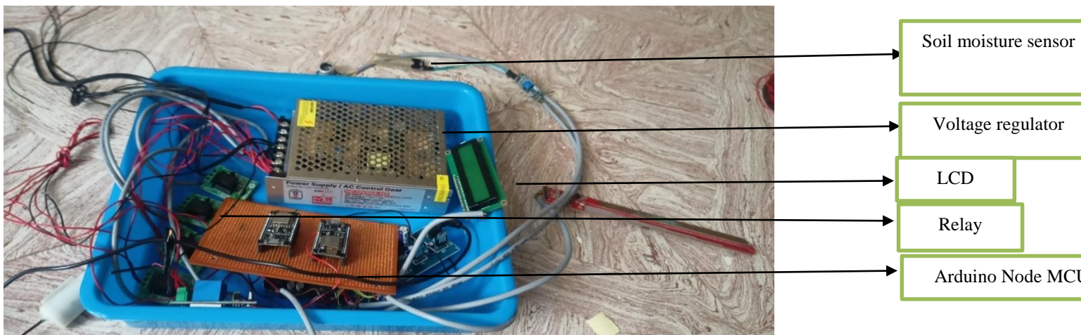
Fig7.1.2 IoT Based Solar powered Fertigation cum Natural Manure(panchagavya) Dispenser
