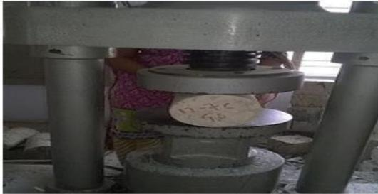
Fig.4.1.split tensile strength test.
