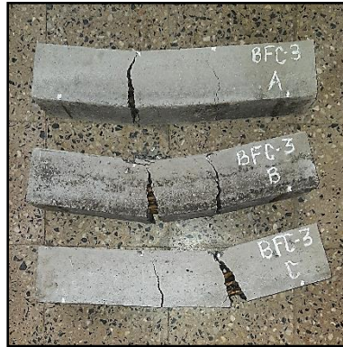
Figure No. 2: Crack pattern in BFC-3 (bamboo mesh) Specimen
