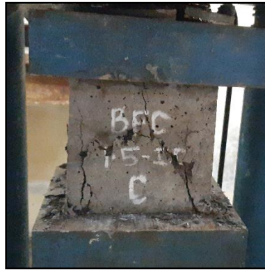
Figure No. 3: Compression failure of Ferrocete Specimen showing delamination
