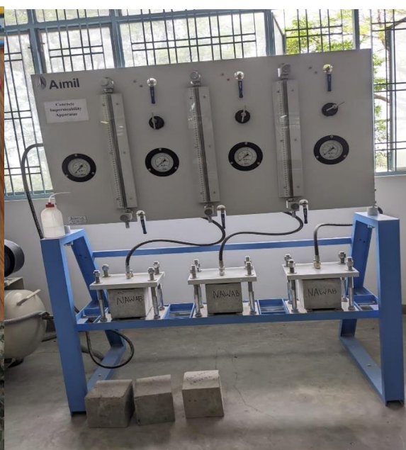
Fig. 12. Water permeability testing
