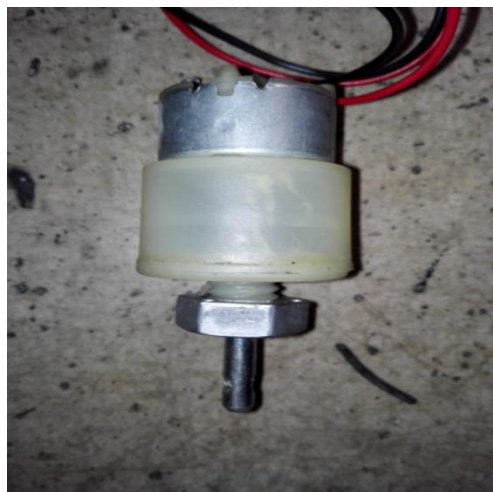
Fig: 12 seed motor roller motor 12 v, 10rpm
