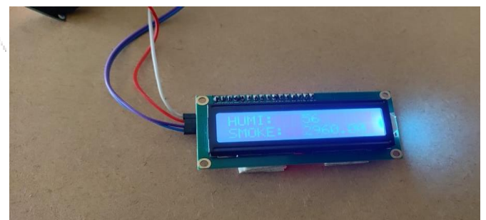
Fig. 9: LCD displaying the smoke value
