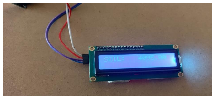
Fig. 11: LCD displaying the soil content value
