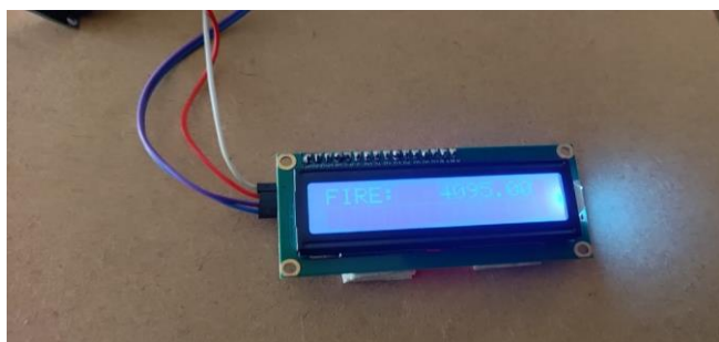
Fig. 7: LCD displaying the fire value
