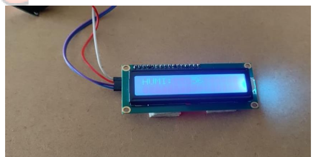
Fig. 15: LCD displaying the humidity value
