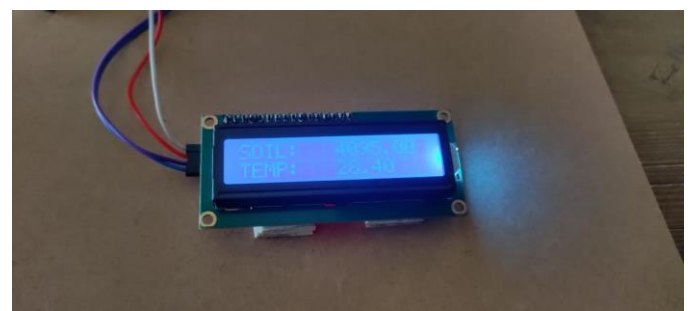
Fig. 13: LCD displaying the temperature value
