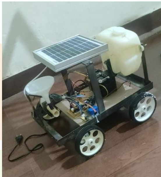
Figure 5.1. Prototype model of Autonomous Agrirobot
