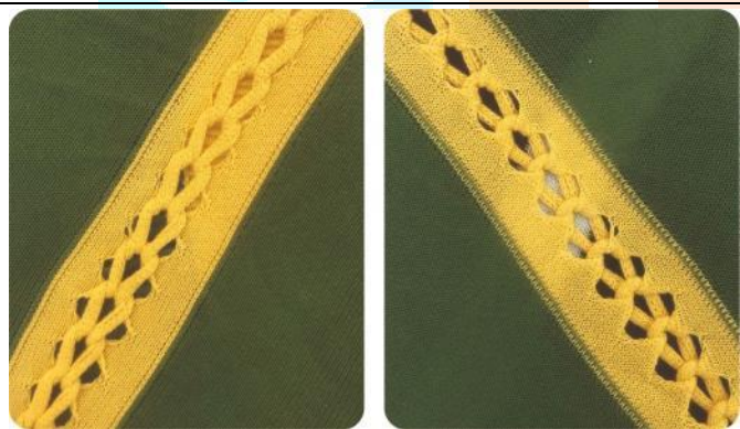
Fabric view: Knit (front side) at left and Pearl (rear side) at right
