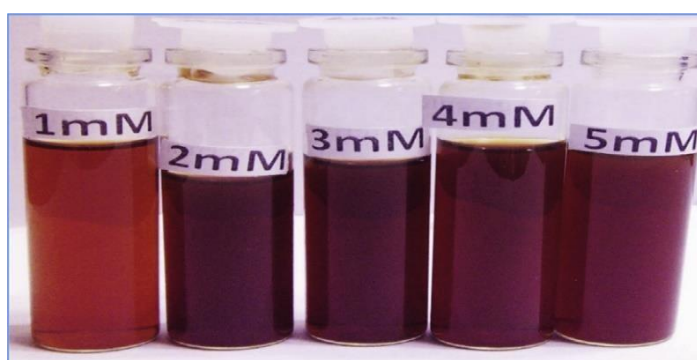
Fig. 1 e Digital optical images of synthesized silver nanoparticles with different conc (1e5 mM) of AgNO 3 .
