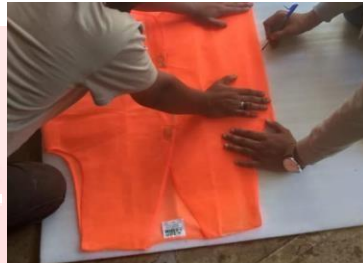
Fig: Marking of the Foam Sheet
