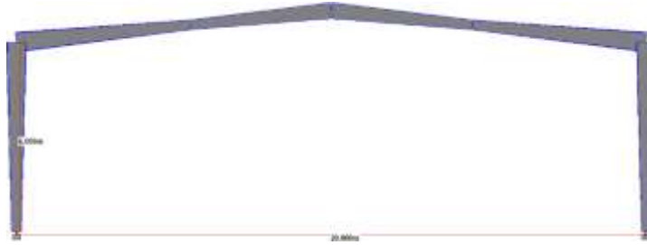
Fig -4: Section of Pre-Engineered Building
