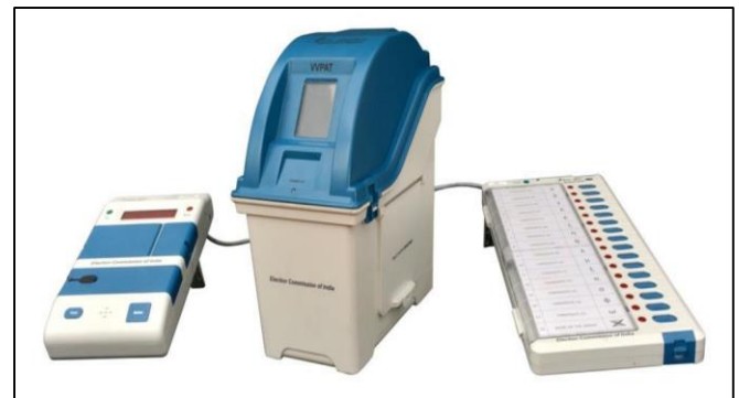
Fig 1: Control Unit, VVPAT Unit, Ballot Unit [5]
