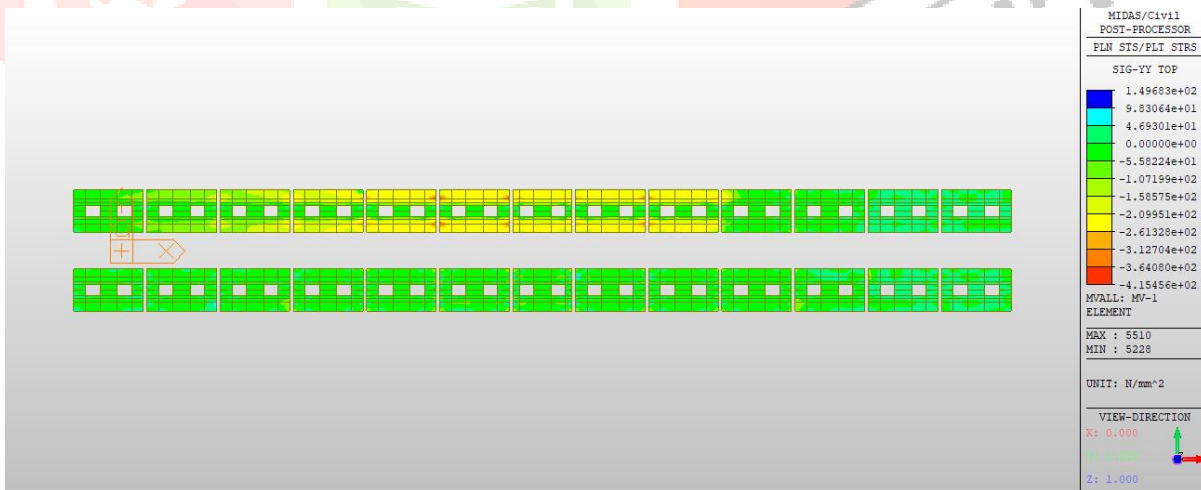
Figure 5b Transverse Stress
