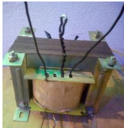
220 TO 12-0-12 TRANSFORMER 5Amp and 14Amp o/p
