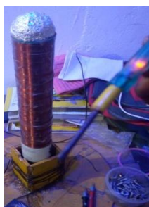
Output of wireless energy system after increasing the power of modulating signal
