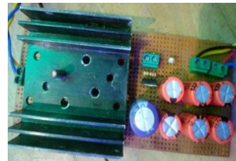
Full wave bridge rectifier OR A.C to D.C Converter
