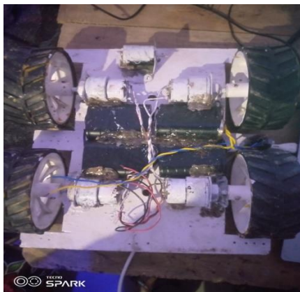
Installing the Motor and battery on the Robot
