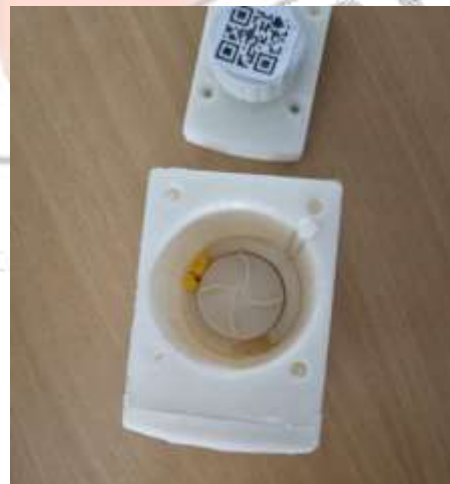
Figure 2 – Pill Dispensing Mechanism placed inside the pill box,
