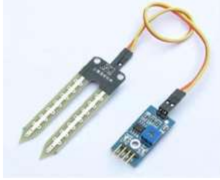
fig 3: soil moisture sensor
