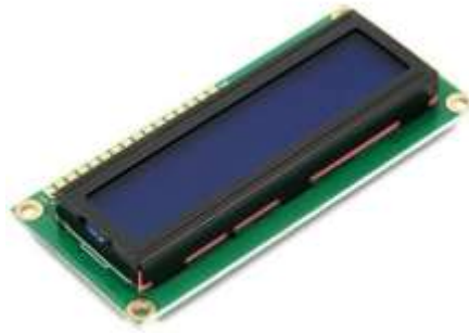
fig 9: i2c 16*2 lcd display
