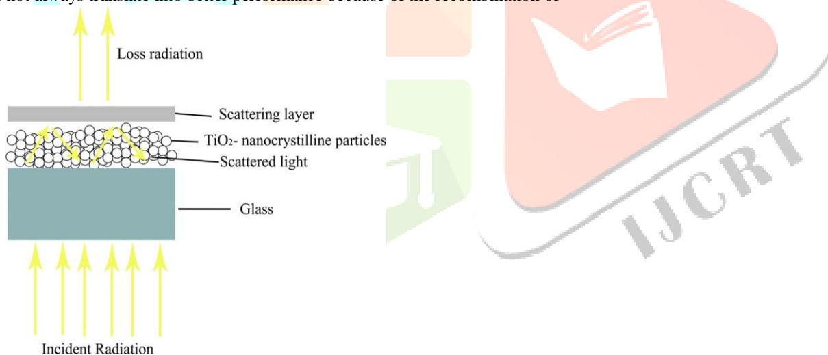
Figure 6: Diagram expresses several layers on top of nanocrystalline TiO 2 and scatter light
