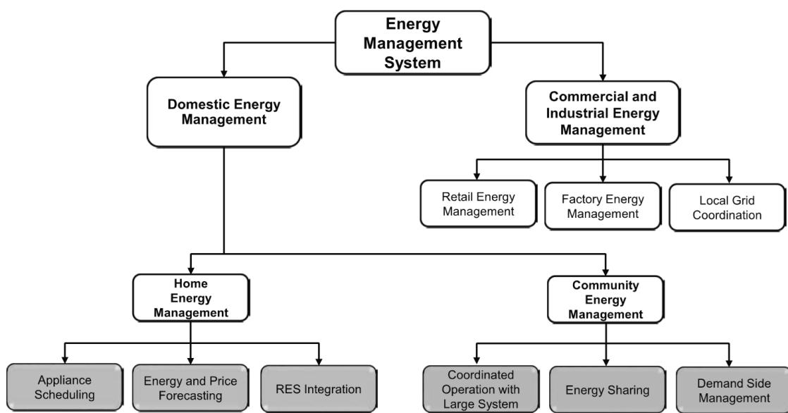
Figure 1. Energy management system in the smart grid system [8].
