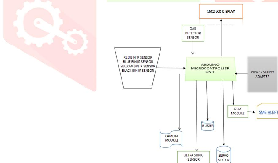
Figure 4.2: Hardware Architecture
