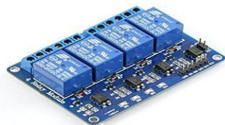
Fig -5: 4-channel relay module
