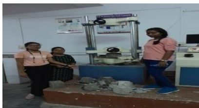
Fig: UTM Testing in Cubes
