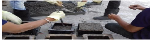
Fig: Fill the concrete in mould &amp; Compacting
