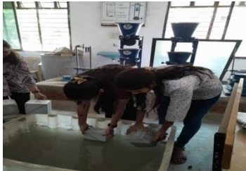
Fig: Curing of Cubes
