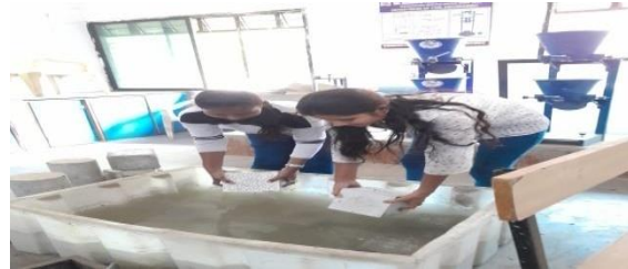
Fig: Curing of Cubes
