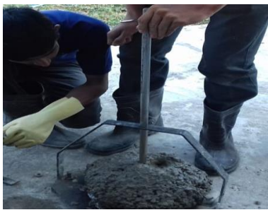
Fig: Collapse Slump Cone
