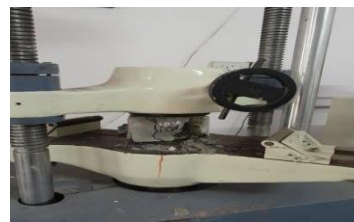
Fig: Cube Testing
