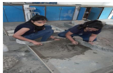
Fig: Hand Mixing of HPC
