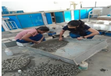
Fig: Hand Mixing of NSC
