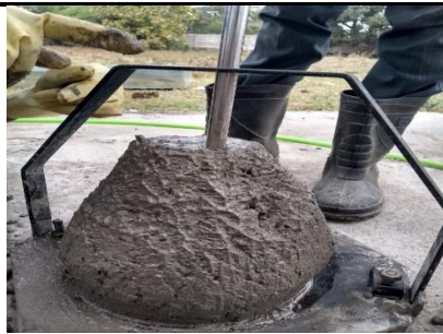
Fig: Collapse Slump Cone
