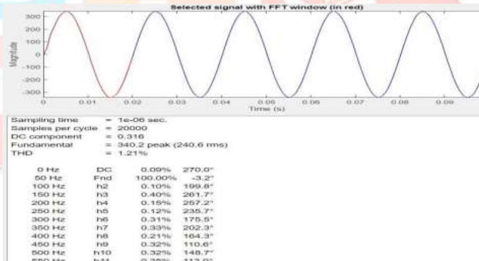
Fig 7.2 : FFT analysis of Output Voltage without grid connection
