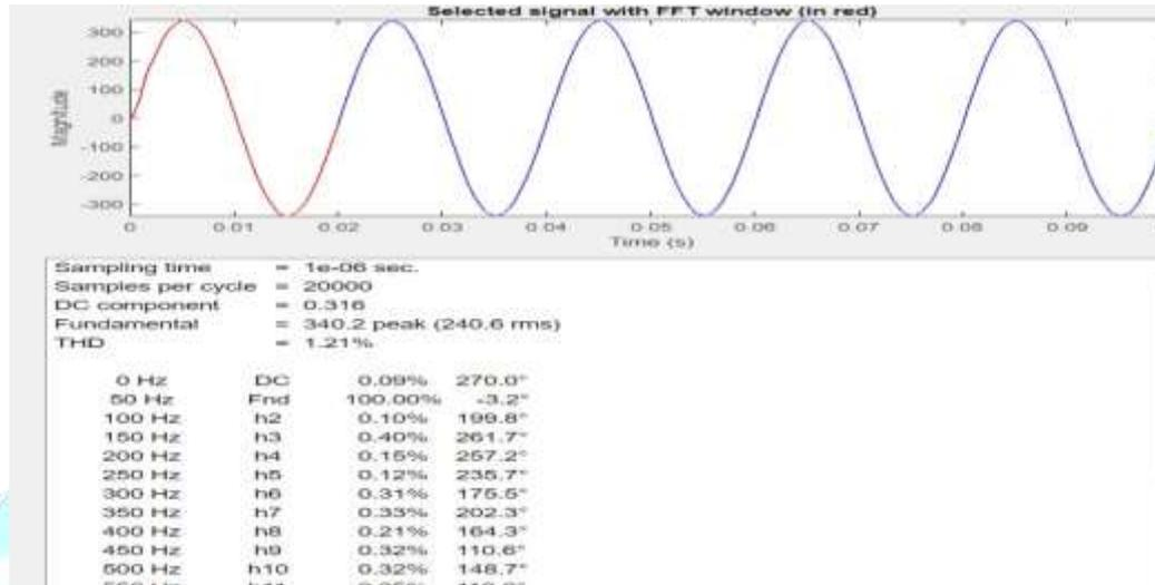
Fig 7.1: FFT analysis of Load voltage with Grid connection
