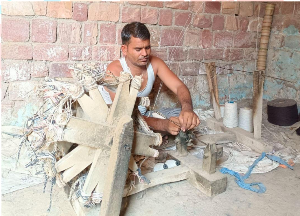
Fig.5: Artisan winding the Bobbins from the spools
