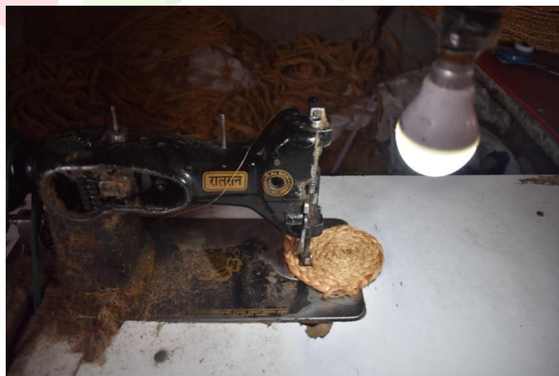
Fig.8: Artisan making the circular Chindi Durri with braided rope.
