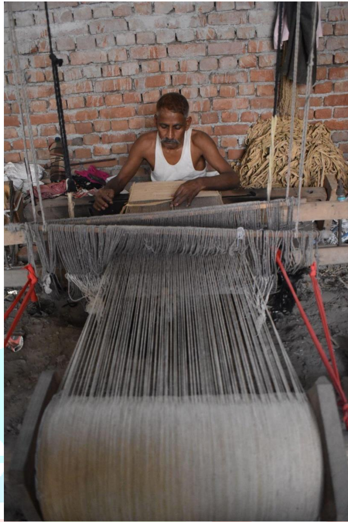
Fig.7: Artisan making the Chindi Durri using Pit loom
