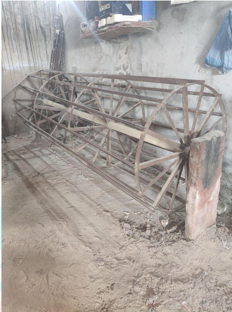
Fig.6: Octangular frame for Warping
