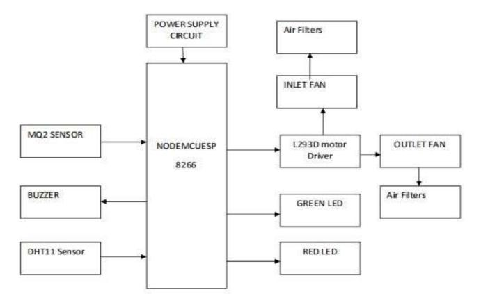
Fig: IoT based air quality monitoring and purification system.
