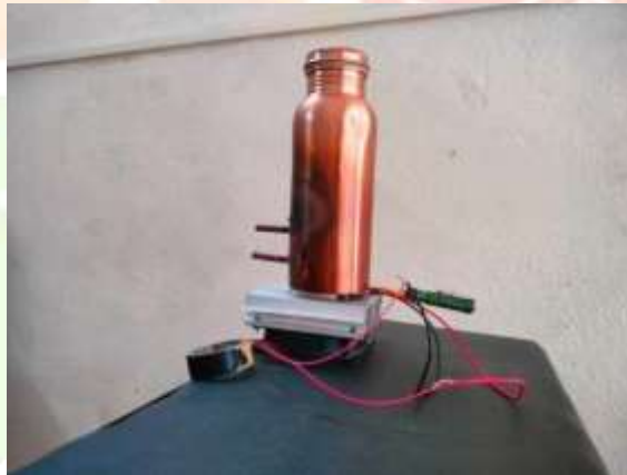
Fig 3.2.3a Coolant storage tank
