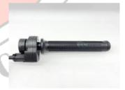
This throttle is technically referred to as a Hall Effect type. The throttle has three wires contains black, red, and green. The supply voltage is via red and black wires and is usually around 4 volts. Green wire voltage increases as the throttle is turned.
