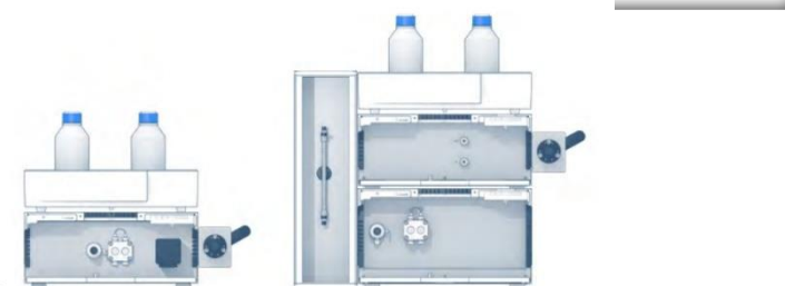
Fig. 4 Isocratic system configuration with a single wavelength UV-detector (left) and a refractive index detector (right)
