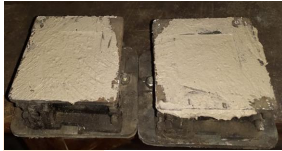
Fig 2.1 Sample for compaction testing
