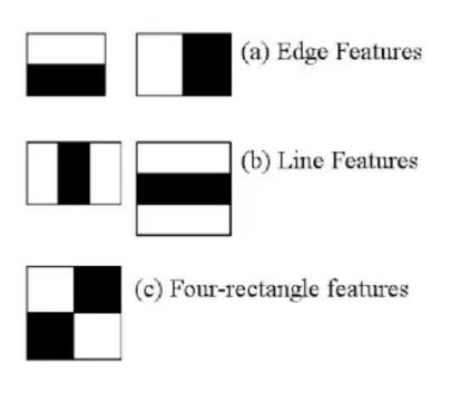
These features can be difficult to determine for a large image. This is where **integral images** come into play because the number of operations is reduced using the integral image.
