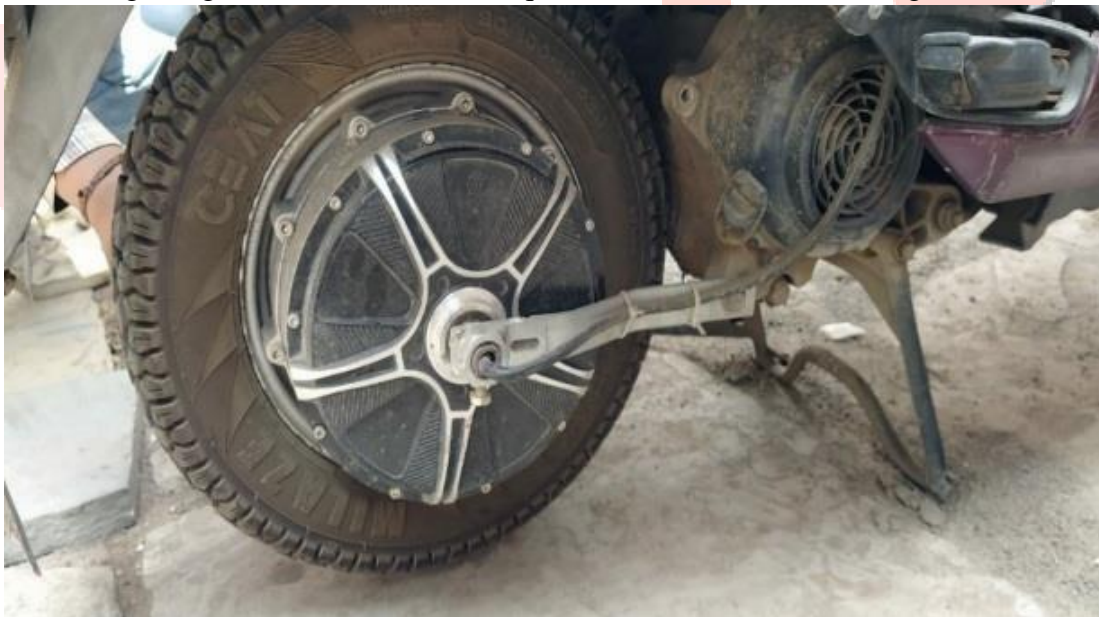
Figure 10. Torque arm and Hub motor fitment
