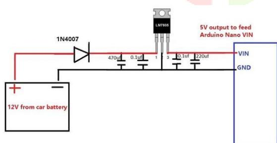
To use the converter, the positive and negative wires from the 12V battery are connected to the input terminals of the converter. The positive and negative wires from the output terminals of the converter are then connected to the device that requires 5V power. It is important to follow the manufacturer's instructions for the specific converter being used and take necessary precautions to avoid electric shock or short circuits.
