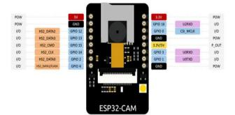
The camera module is connected to the ESP32 via a standard SPI interface, requiring a minimum of 4 GPIO pins for operation. It also includes an SD card slot for storing images and video. The module can be powered using a 3.3V power supply and consumes approximately 100mA of current during operation. It also includes a sleep mode for low power consumption when not in use.
