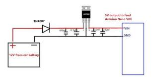
To use the converter, the positive and negative wires from the 12V battery are connected to the input terminals of the converter. The positive and negative wires from the output terminals of the converter are then connected to the device that requires 5V power. It is important to follow the manufacturer's instructions for the specific being converter used and take necessary precautions to avoid electric shock or short circuits.
