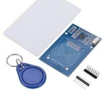
The RC522 RFID reader includes built-in security features, such as a 48-bit unique ID number for each device and support for encryption and authentication protocols. These features ensure the security and privacy of the data stored on the RFID tags and prevents unauthorized access to the system.
