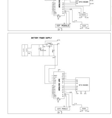
in its path. The NodeMCU will act as the main controller to collect data from all sensors and control the trolley's movement. The Arduino Uno will be used to control the four BO motors that drive the trolley. A WIFI module will be used to communicate with the trolley from a mobile application. A buzzer will provide audio feedback to the user, and an LCD will display the product information and billing details. The webserver will store all transactional data and generate bills automatically.
