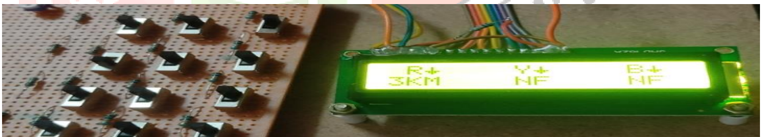
Fig:-LCD displaying fault in Red cable at a distance of 3km
