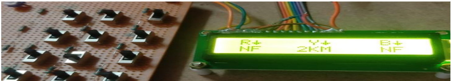
Fig:-LCD displaying fault in Yellow cable at a distance of 2km
