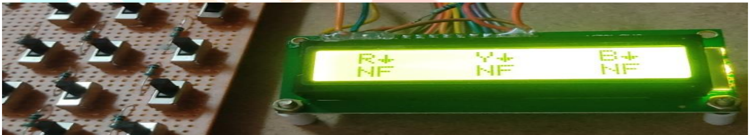
Fig:- LCD displaying No Fault
