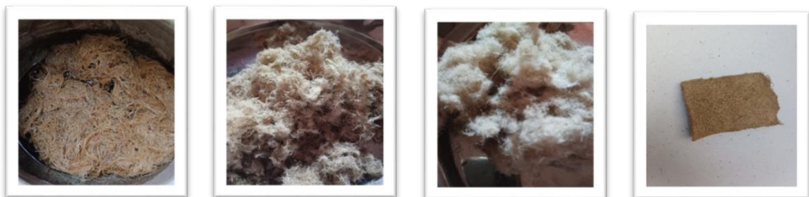
(Plate3:fibre build with (Plate4:semi dried fibre) (Plate5:fluffy fibre) (Plate6:non-woven core NaOH ) material)
