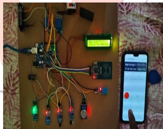
Figure(4.2). Implementation of Vibration detection using Blynk app
