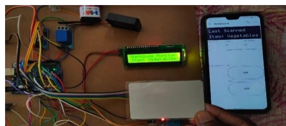
Figure (4.6.1). Implementation of Vegetable detection using Blynk app
