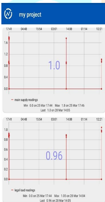
Fig-7.1: Results during legal load only (1.0 is the reading of main supply(cs1) and 0.96 is the reading of legal load(cs2))
