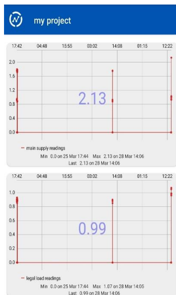
Fig-8.1: Results during legal load only (1.0 is the reading of main supply(cs1) and 0.96 is the reading of legal load(cs2))
