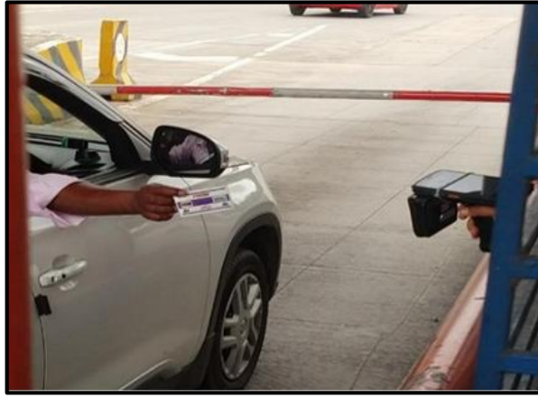
Figure 3: Tag not attached to the windshield.
