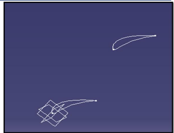
Figure 3: NACA 6409 airfoil with distance 49.2mm (9)
