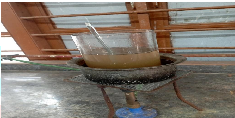
Figure 6 : In preparation of nanocellulose – the mixture was heated at 50 °C for 2 h
