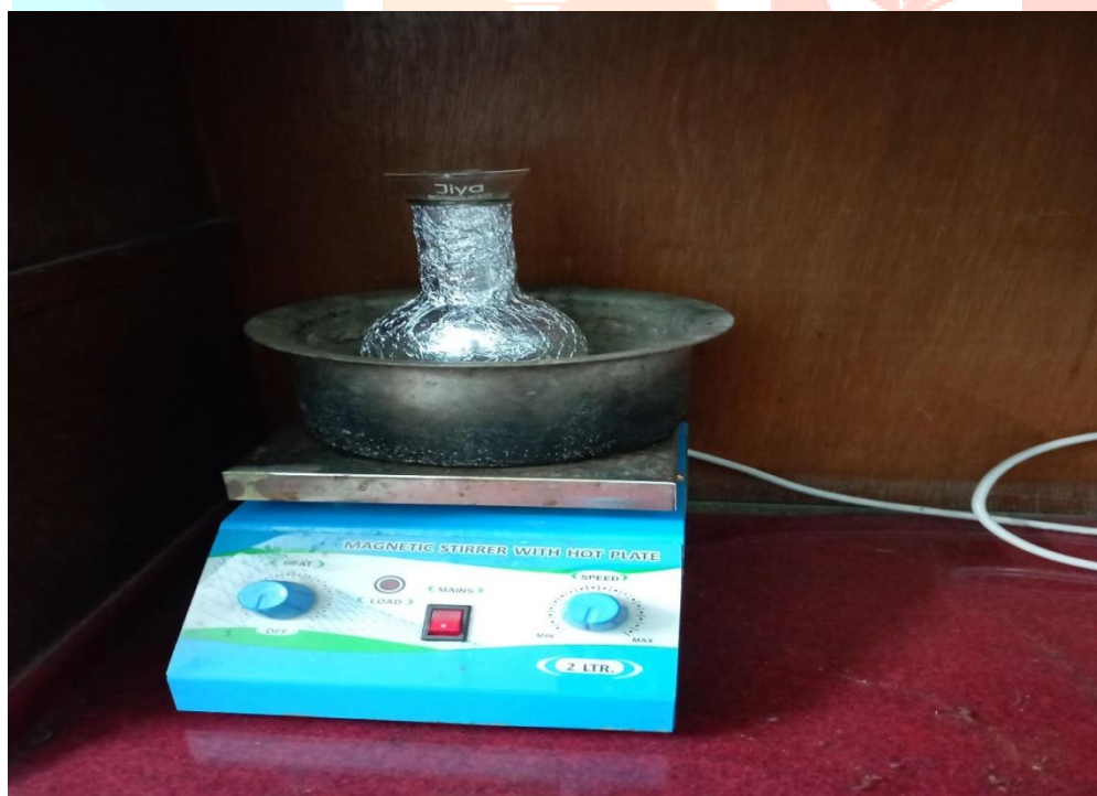
Figure 10 : Synthesis of folic acid conjugated NC – Stirred overnight
