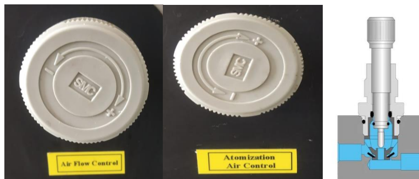
Fig. Control Switch For Inlet Airflow And Atomization Air
