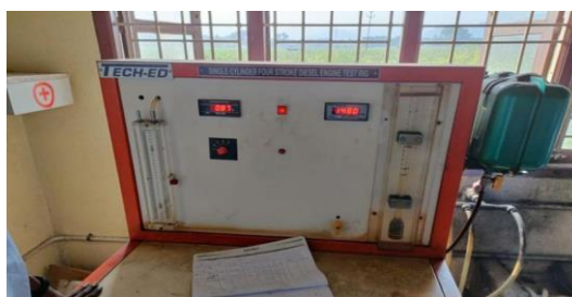
Fig : 4 Single Cylinder Four Stroke Diesel Engine Test Rig (without Turbo charger)
