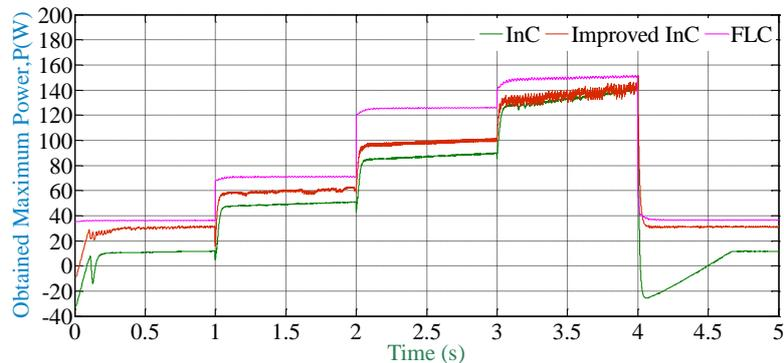
Fig.11:OMP with the InC and improved InC algorithms under both the variations of the solar irradiation and temperature
