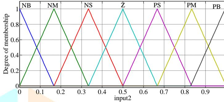
Fig. 5: Triangular MF of input2
