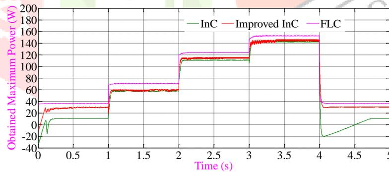
Fig.9:OMP with the InC and improved InC algorithms under the variation of the solar irradiation
