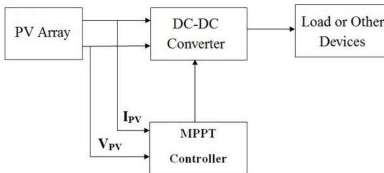
Fig.2: Block diagram of MPPT
