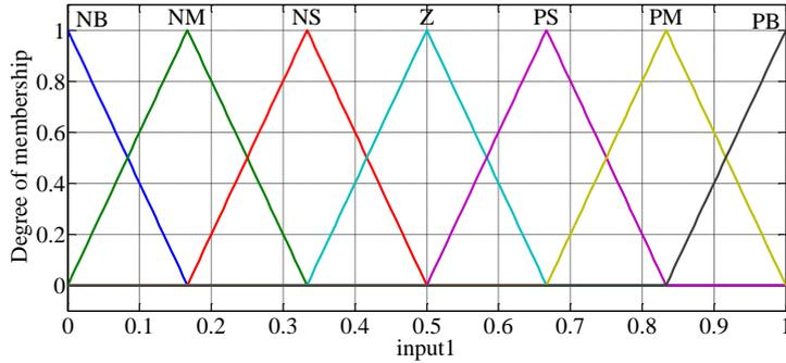
Fig. 4: Triangular MF of input1
