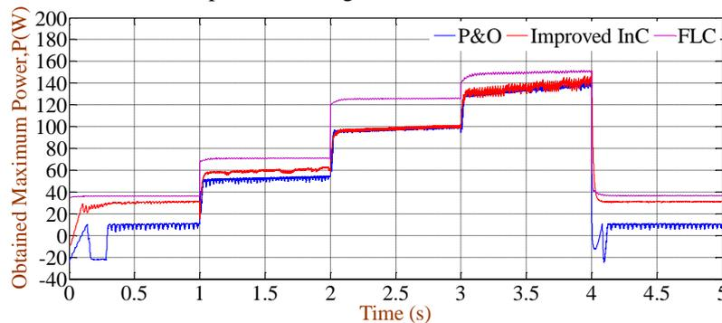
Fig.10:OMP with the P&O and improved InC algorithms under both the variations of the solar irradiation and temperature
