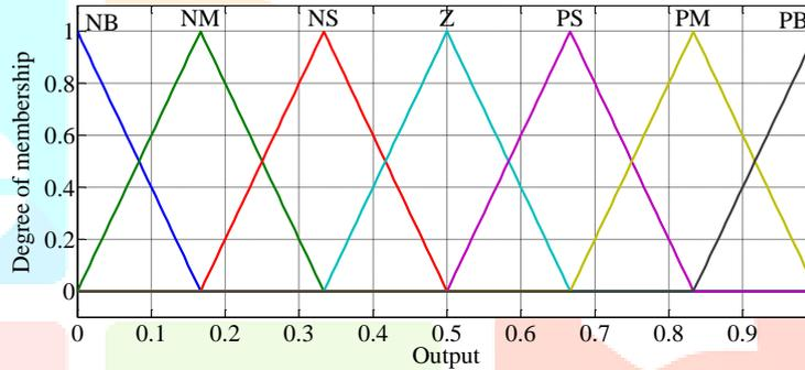
Fig. 6: Triangular MF of output
