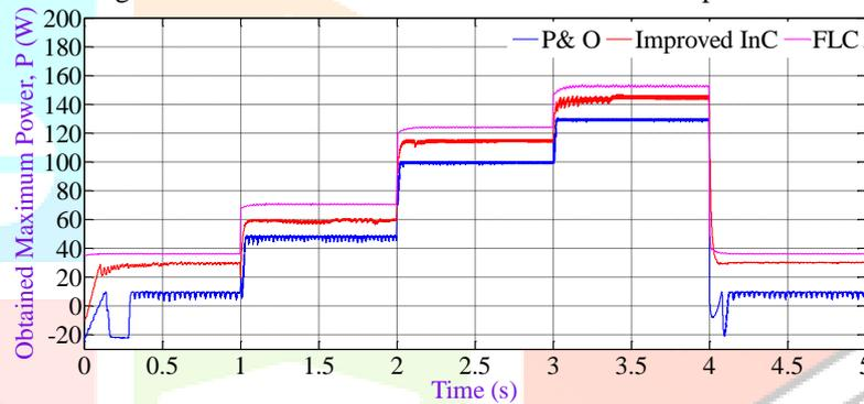
Fig.8:OMP with the P&O, improved InC algorithms and FLC under the variation of the solar irradiation
