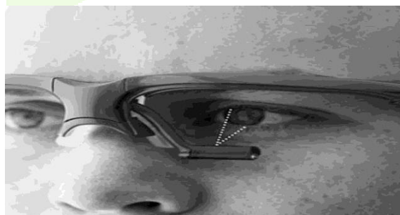
Fig-4: A pictorial representation of Infrared Oculography
