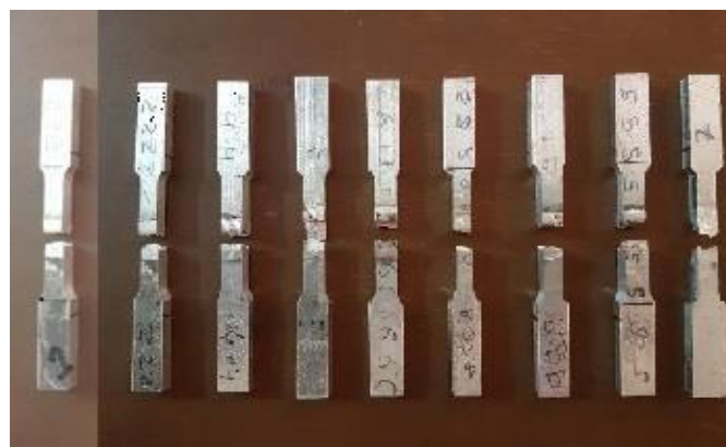
Figure 9. Tensile specimens after tensile testing
