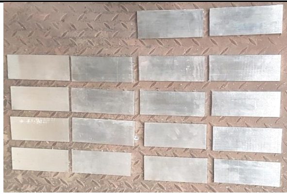
Figure 2. Sheared pieces of AA 7075 Sheet material
