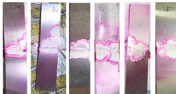
Figure 4. Dye penetrate test samples 1
