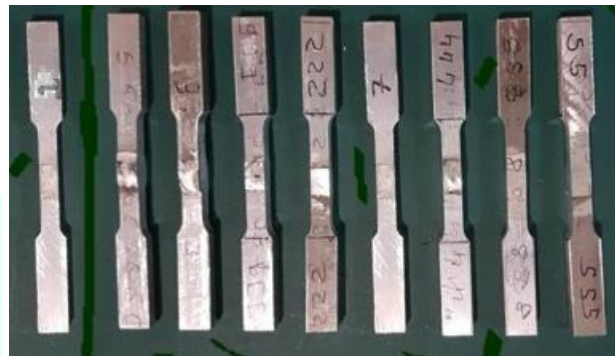
Figure 8. Prepared tensile specimen as per ASTM E8Standard
