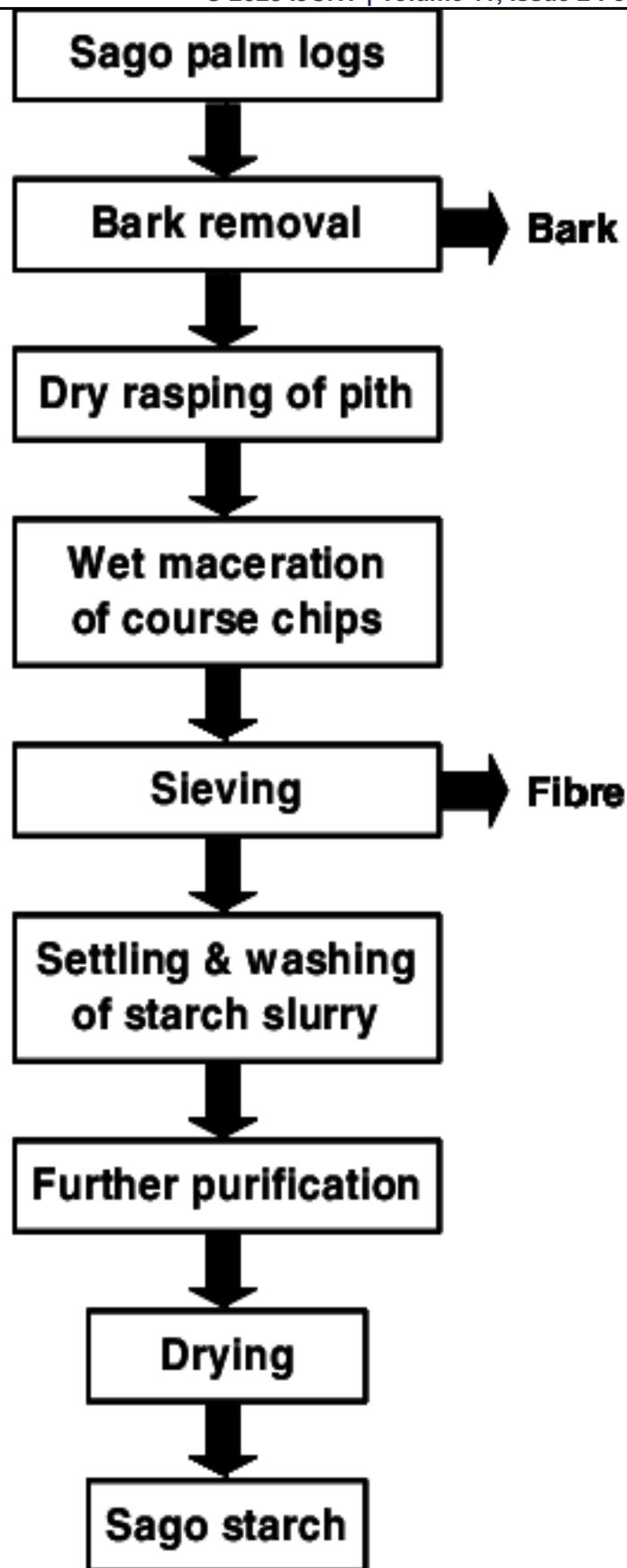
Fig (4) Production of Sago Starch
